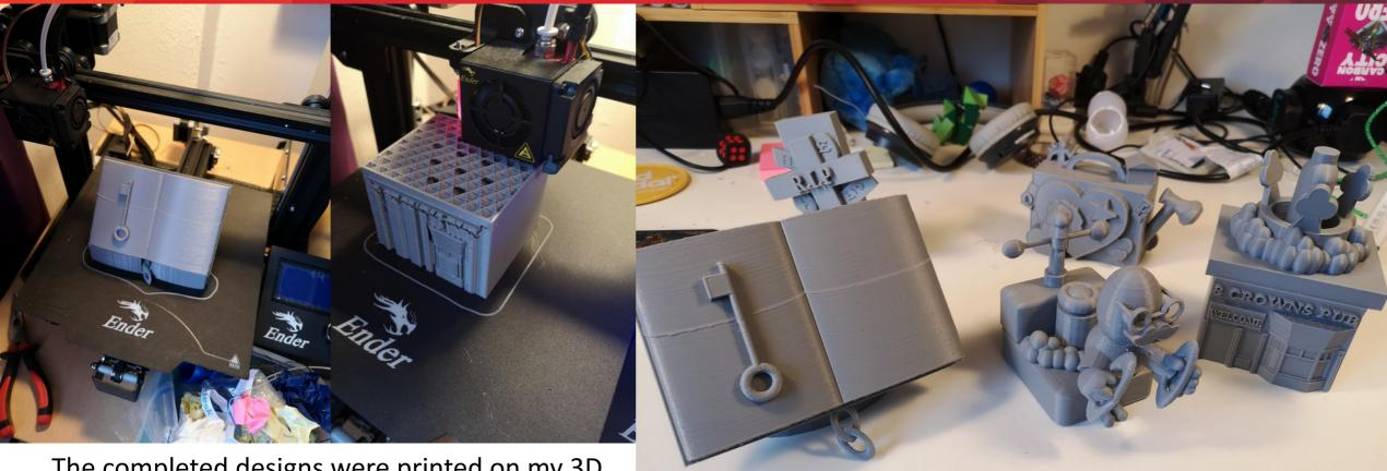
The completed designs were printed on my 3D printer before being sanded, primed and painted to look like antique metal.
